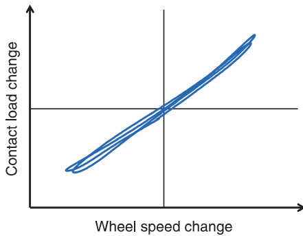
Fig. 4 Relationship between change in wheel speed and change in tire contact load for front wheel
